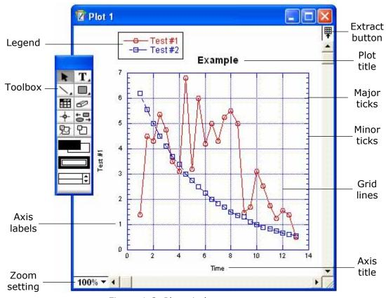
Figure 1-3 Plot window components
