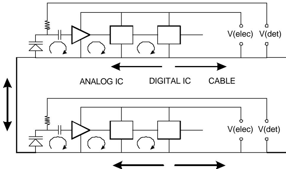
Since the cross-connection at the input is formed by the connection of multiple chips to the detector, it is unavoidable.
