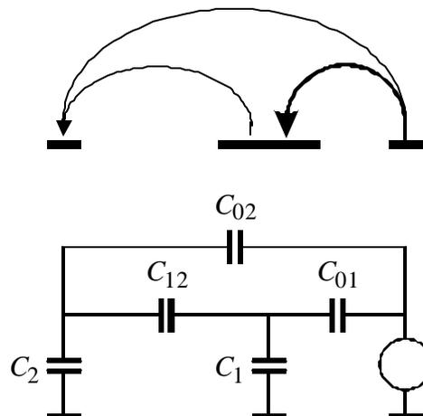
“Field line pinning” is the operative mechanism of “Faraday shields”.
