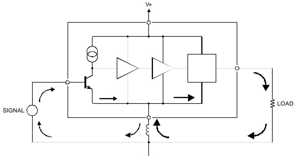
The output current is typically orders of magnitude greater than the input current (due to amplifier gain, load impedance).
