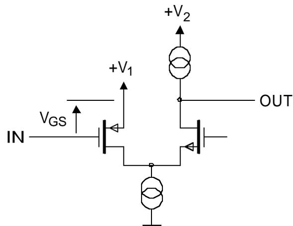
The problem with this configuration is that the supply  $V_1$  becomes part of the input signal path. Unless the  $V_1$  supply bus is very carefully configured and kept free of other signals, interference will be coupled into the input.
