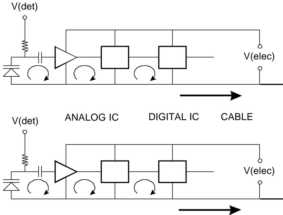
Since the path of least resistance is provided by the cabling and connections to the power supplies and data acquisition system, current transients originating in the front-end circuitry do not flow towards the input.
