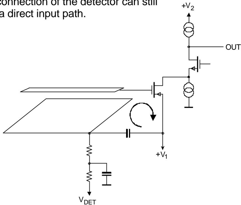
In most implementations supply lines are more susceptible to pickup, so the  $+V_1$  line must be properly filtered to prevent current injection.
