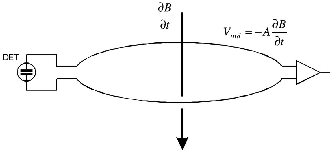
Clearly, the area  $A$  enclosed by any loops should be minimized.
