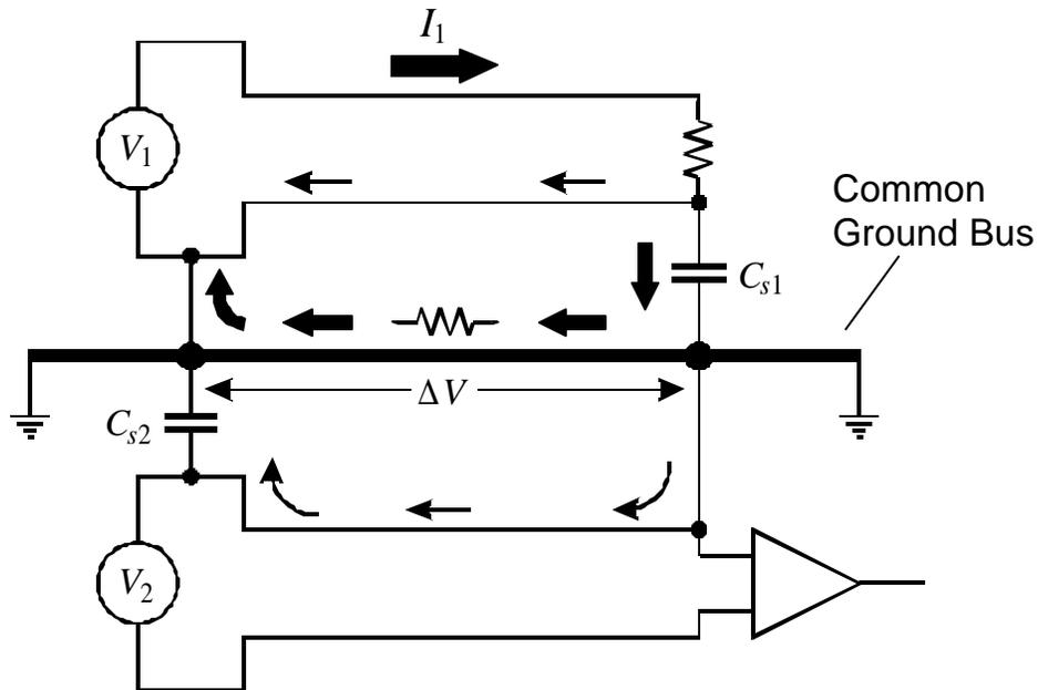
The loops in this figure are the same as shown before, but the loops are closed by the capacitances  $C_{s1}$  and  $C_{s2}$ . Frequently, these capacitances are not formed explicitly by capacitors, but are the stray capacitance formed by a power supply to ground, a detector to its support structure (as represented by  $C_{s2}$ ), etc. For AC signals the inductance of the common current path can increase the impedance substantially beyond the DC resistance, especially at high frequencies.
