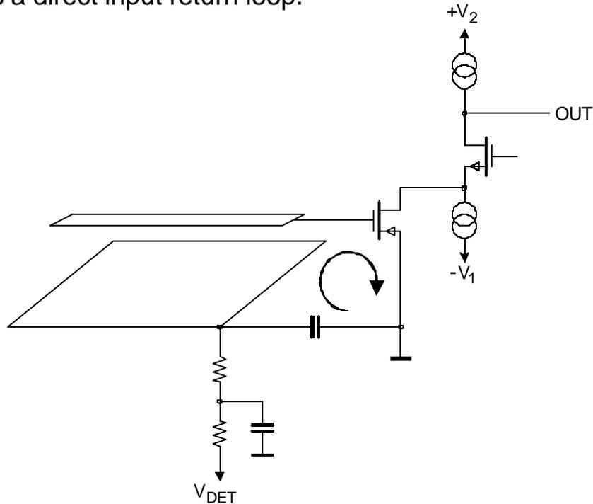
For some (mythical?) reason positive supplies are more popular. Proper connection of the detector can still provide a direct input path.
