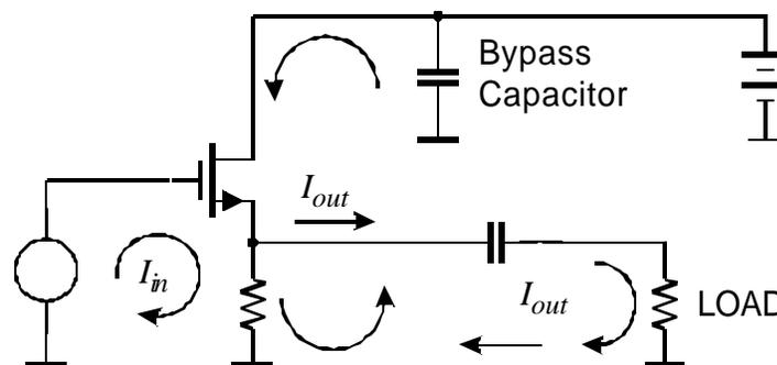
Since the “ground” is a large area conducting surface – often a chassis or a ground plane – with a “low” impedance, it is considered to be an equipotential surface.
