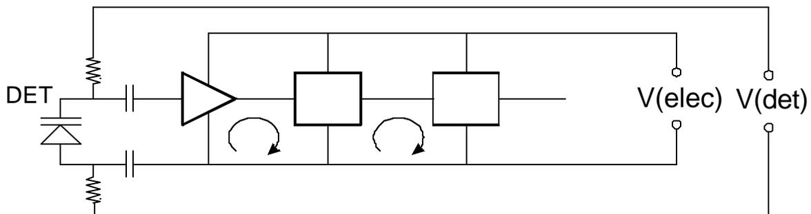
The resistors in both legs of the bias connection isolate the sensitive input node by presenting a high impedance to external signals. Only one of the two capacitors at the input may be necessary, depending on system requirements.
