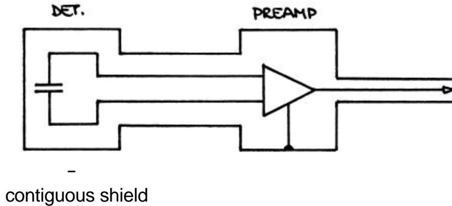
Conducting shield attenuates an incident electromagnetic wave because of
