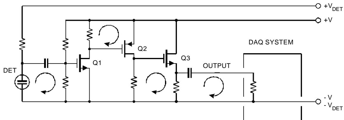
In transferring from stage to stage the signal current flows through local return loops.
