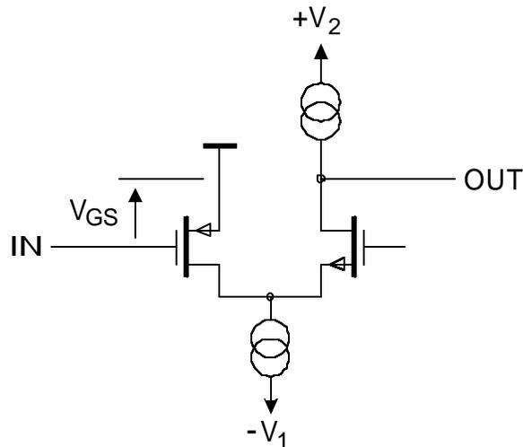
Connected to a strip detector (and redrawn slightly), this configuration provides a direct input return loop.
