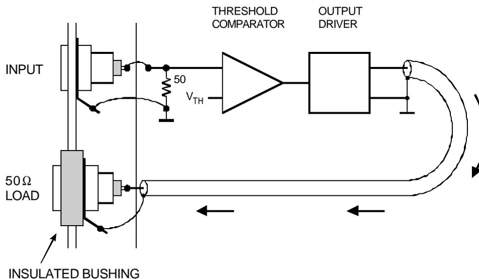
Often it is convenient to replace the coax cable at the output by a strip line integrated on the PC board.
