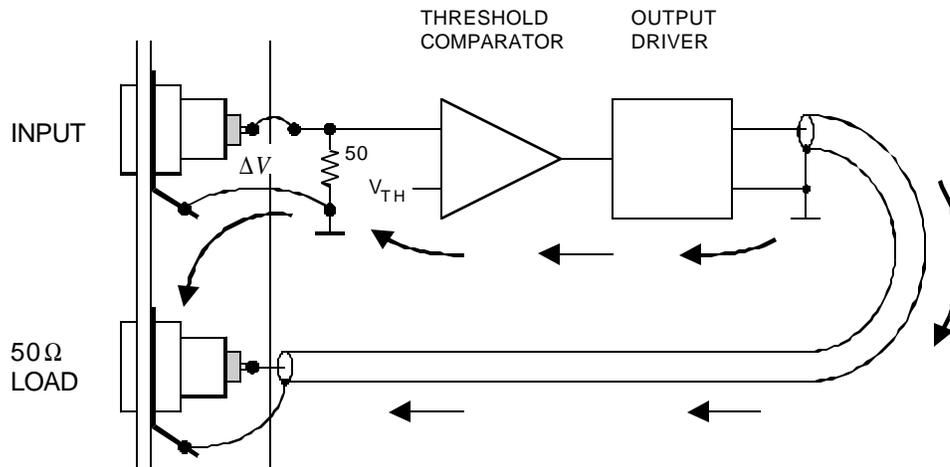
A portion of the output current flowed through the input ground connection. The voltage drop  $\Delta V$  was sufficient to fire the comparator.
