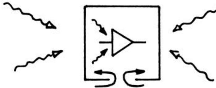
External fields can penetrate significantly if openings  $> \lambda/1000$  (diameter of holes, length of slots).
