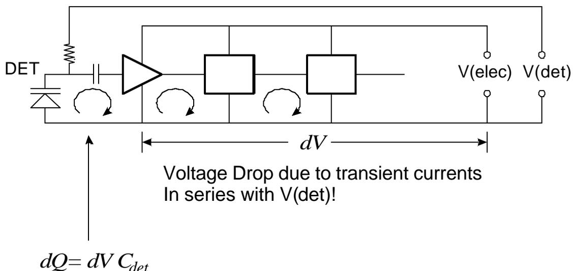
The transient voltage drop  $dV$  is superimposed on the detector bias and injects a charge  $dQ = dV C_{det}$  into the input.
