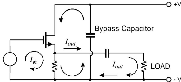
In addition to the signal currents  $I_{in}$  and  $I_{out}$ , the drain current is also changing with the signal and must return to the source. Since the return through the power supply can be remote and circuitous, a well-defined AC return path is provided by the bypass capacitor.
