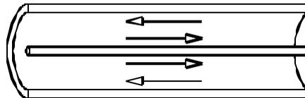
Net field at *outer surface* of shield is zero.
