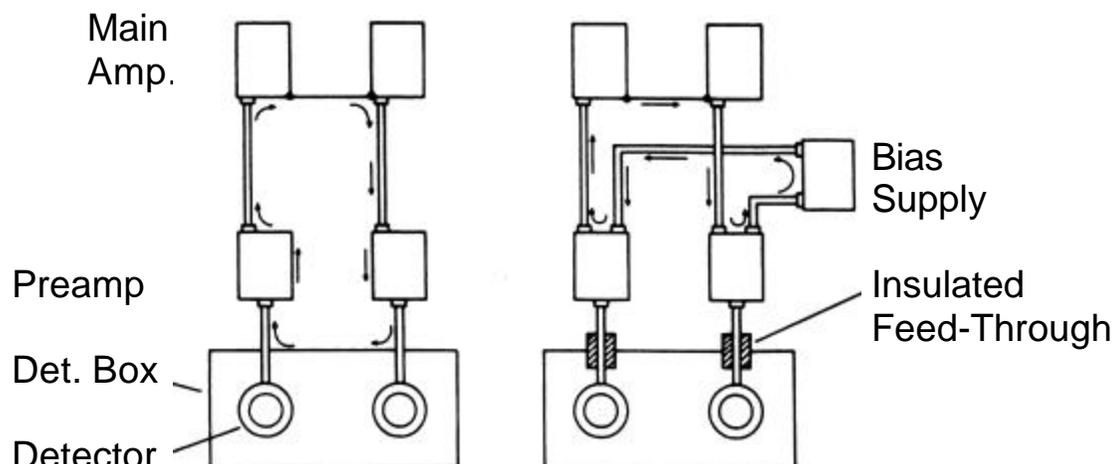
The configuration at the left has a loop that includes the most sensitive part of the system – the detector and preamplifier input.
