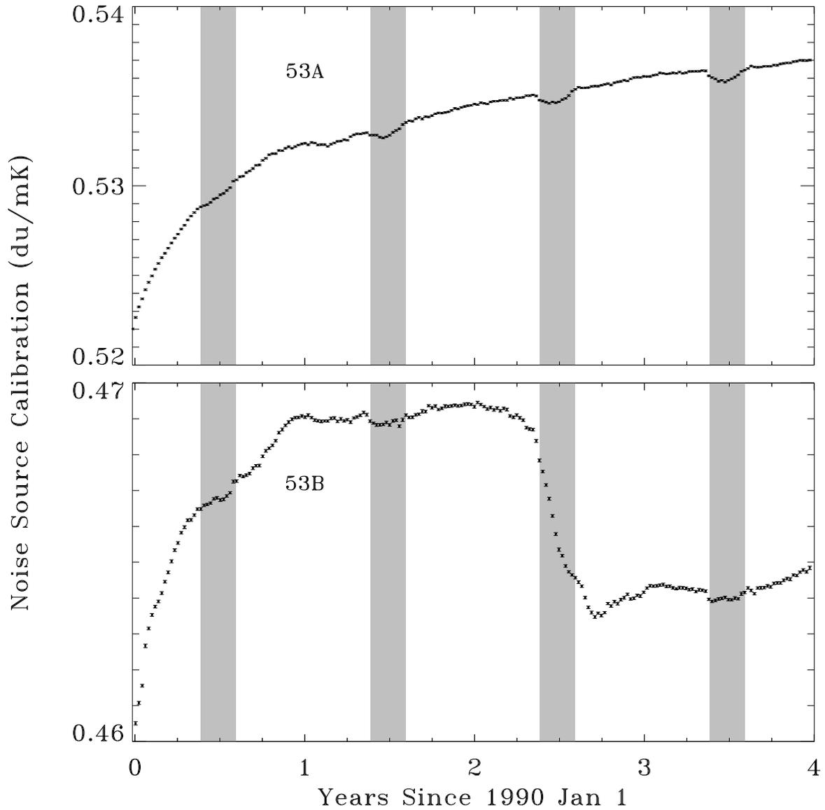
Figure 5: Calibration factor  $\mathcal{G}'(t)$  derived from on-board noise sources for the 53A and 53B channels. Each datum represents one week. The gray bands show the “eclipse season” surrounding the June solstice. The gain is stable to better than 3% throughout the 4-year mission.
